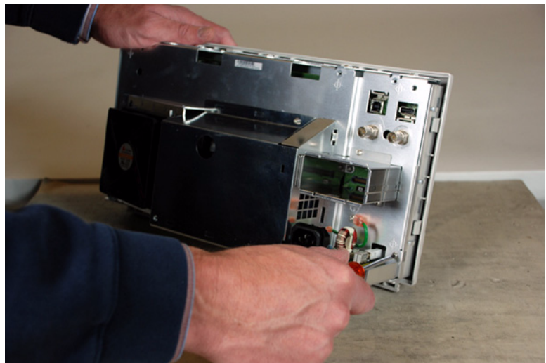
Figure 29 Removing the bottom right rear deck screw
