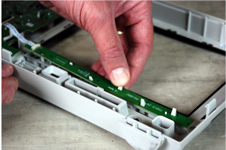
Figure 48 Unclip the softkey board from the bezel
