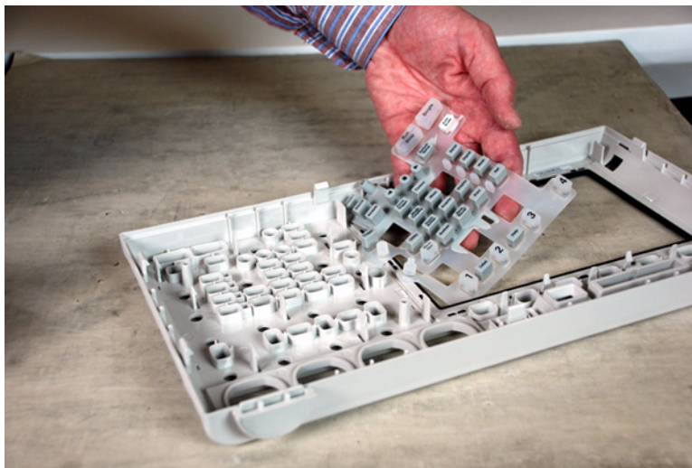
Figure 51 Remove the keyboard keypad from the bezel
