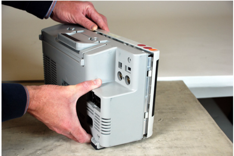
Figure 23 Removing bucket assembly
