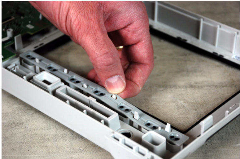
Figure 49 Remove the softkey keypad from the bezel
