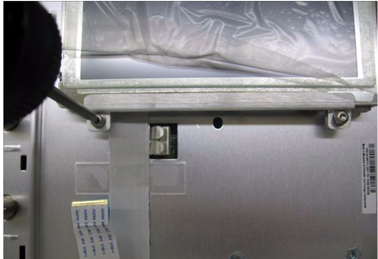
Figure 54 The 75019-68712 display assembly has a bracket under two of the retaining screws
