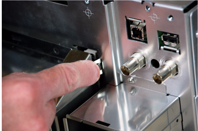
Figure 25 Unclipping the power supply shield right side
