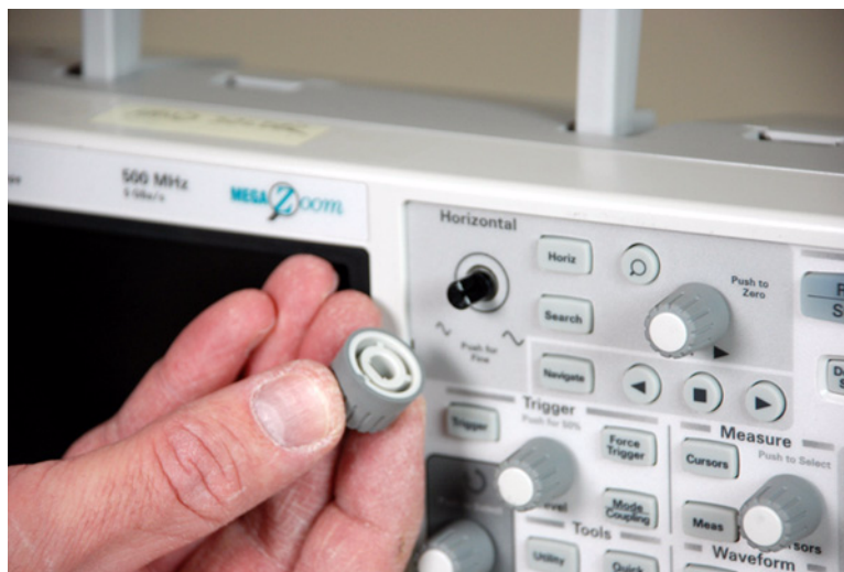
Figure 21 Removing the front panel knobs
