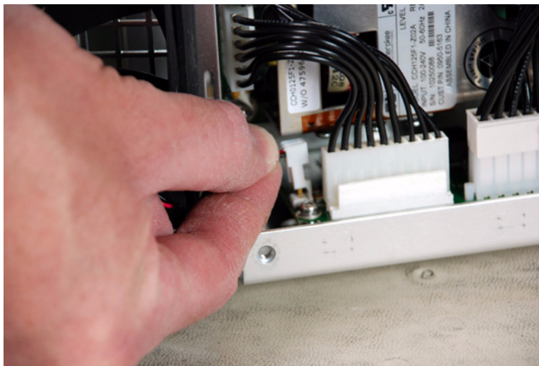
Figure 58 Disconnecting fan power cable
