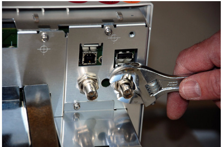
Figure 27 Removing the BNC nuts and washers
